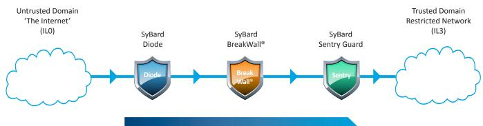
Deep content inspection of data with enforced one-way flow and network-layer to application-layer protocol break
